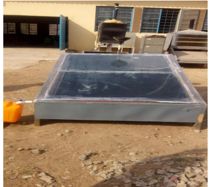
Plate 1: Experimental setup of the constructed optimized solar still.
